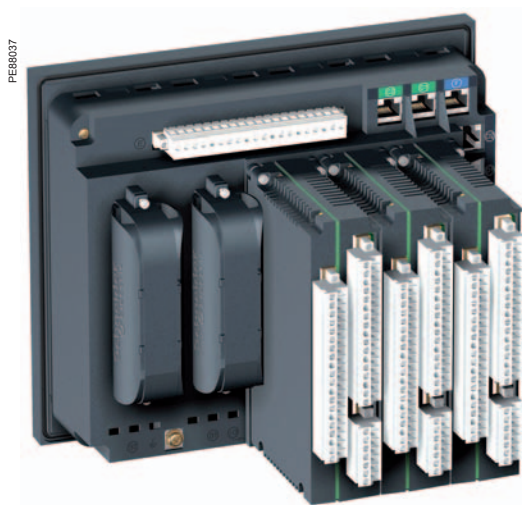
Maximum Sepam series 80 configuration with 3 MES120 modules: 42 inputs and 23 outputs.
