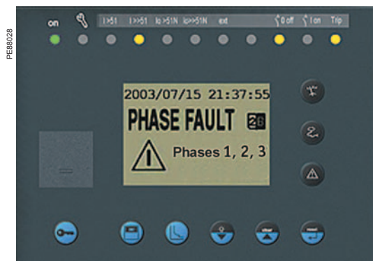
Local indications on the Sepam front panel.
